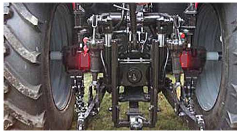
PTO modes: 540/1000 / Ground Speed / Disengage
