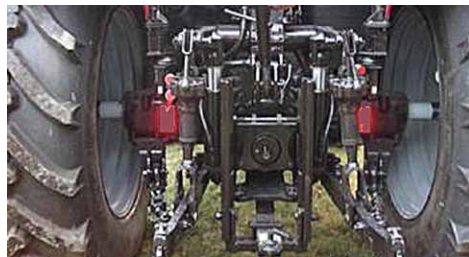
PTO modes: 540/1000 / Ground Speed / Disengage
