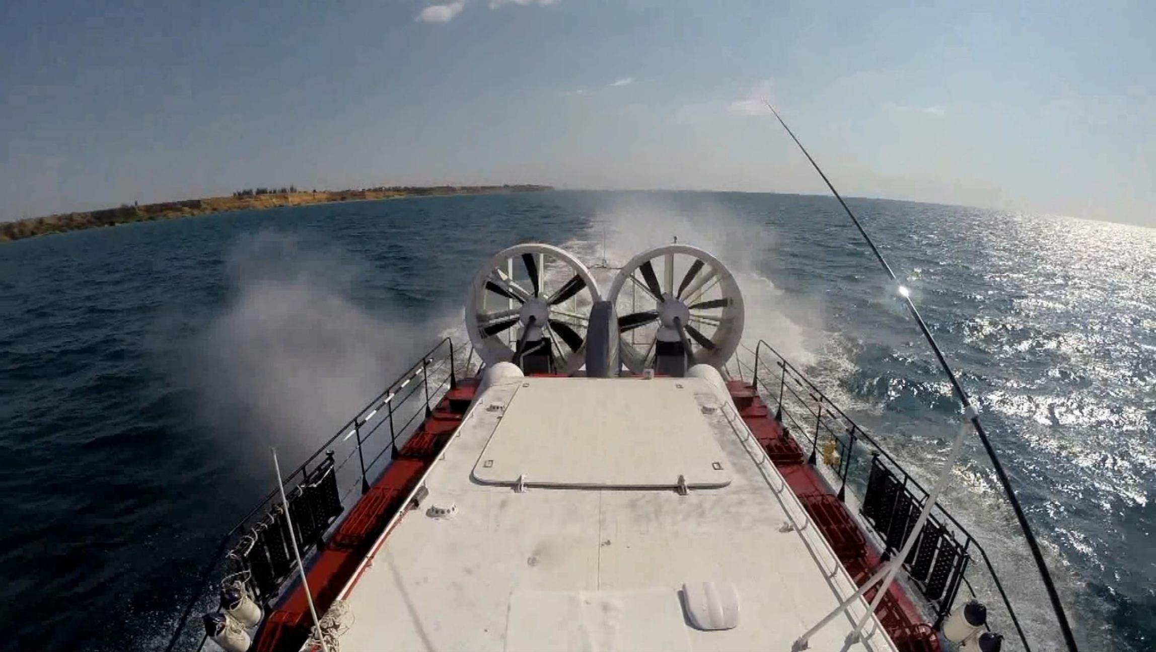
Hovercraft is operational in stormy water up to 4<sup>th</sup> degree (1.25-2.5 m waves).
