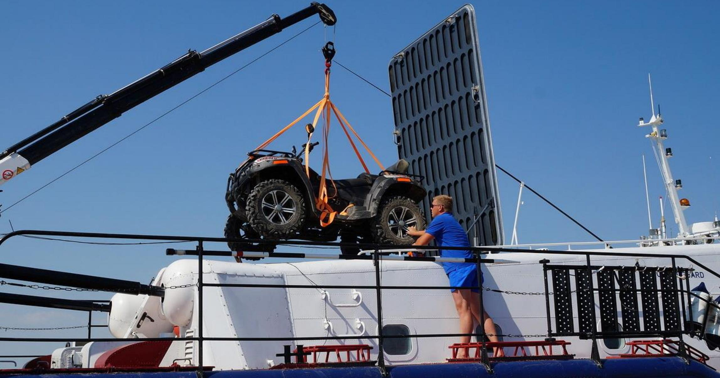
Loading and unloading cargo up to 500 kg using onboard crane / manipulator
