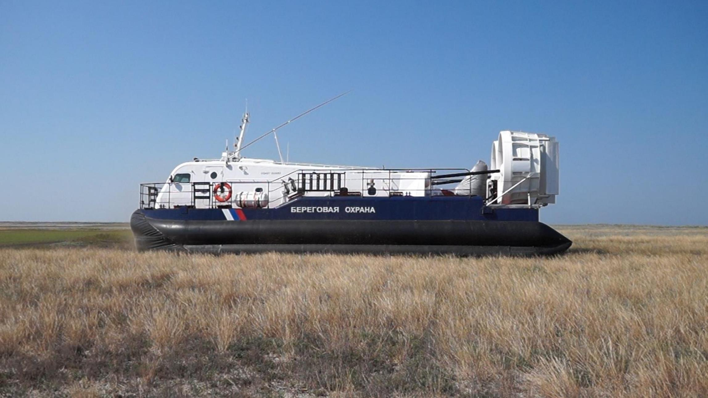
Amphibious capacity of the hovercraft allows no loss of carry capacity overland. Can hover over obstacles up to 1.25 m tall.
