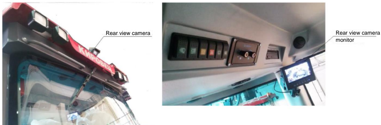
Fig. 9 Location of the rear view camera
