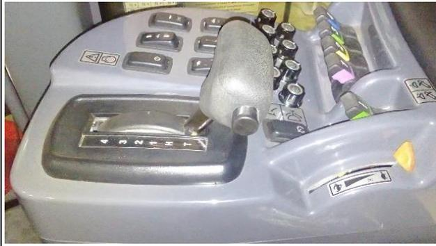
9. Engage a low mode with the use of PVR-1 key by turning lever B counter-clockwise to the fixed position III.
