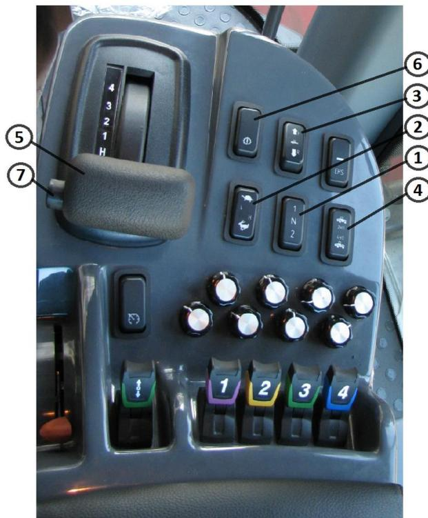
Gears are changed by the lever via cable drive. Lever (5) shall be shifted to position "T" (synchronizing brakes are on) only with retainer 7 pressed.
