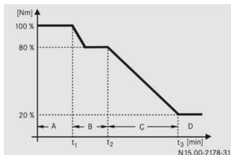
Insufficient AdBlue®/DEF remaining; warning and length of operating restriction period (example display)
