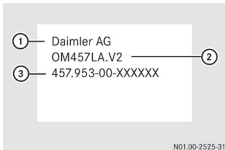
Example: engine data plate for road vehicles (on-highway engine)
