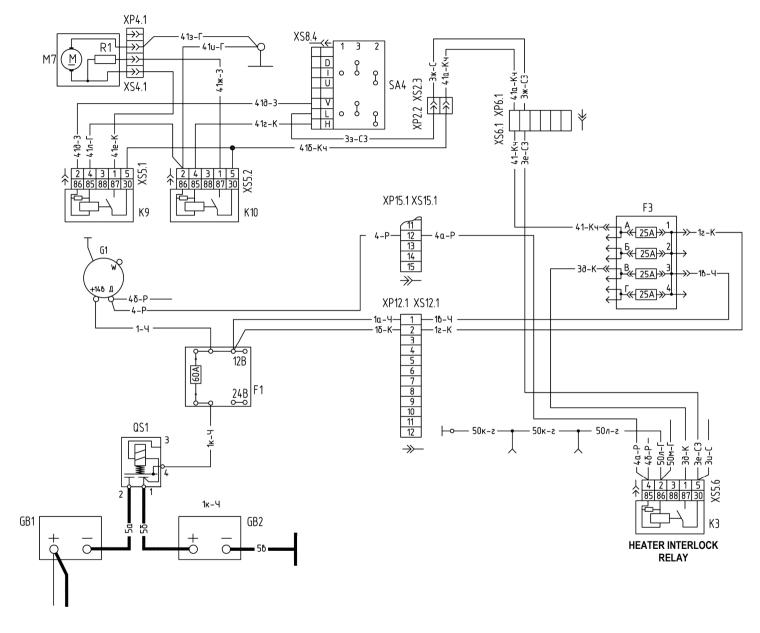
Connection diagram of the cab heater and fan with the fan motor power of 120 W  $_{\rm 240}$
