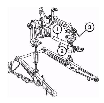
The machine (implement) is also attached to the tractor by the automatic hitch CA-1 connected to the tractor hookup at three points (two rear joints of longitudinal rods and rear joint of the central rod).
