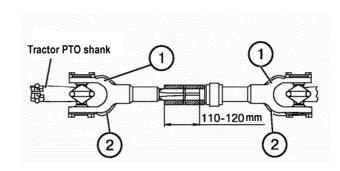
e) having installed the driveline, make sure that the components of the driveline telescopic connection do not abut during extreme machine positions relative to the tractor; the minimum overlap of the driveline telescopic connection shall be 110-120 mm, because lower overlap value could cause the transmission disconnection.
