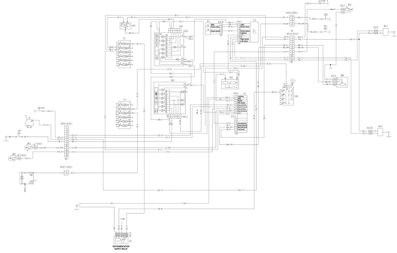
Diagram of the instrumentation dashboard 80-3805010-Д1
