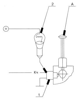
Fig. 7. Checking the operation of the starter interlock switch.
