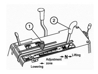
At the beginning of each run, lower the implement by pushing the handle (2) forward to the stop against limiter (1).
