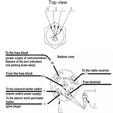
Fig.8. Checking the operability of the starter switch (SA6). For the instrumentation dashboard 80-3805010-Д1.
