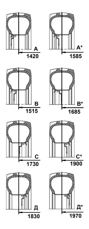
A, B, C,  $\square$  – standard fitting of the disk with transposing the rim;
