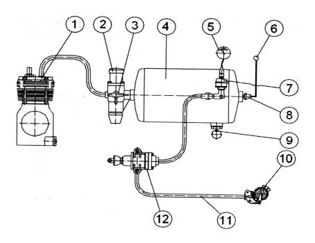
1 – compressor; 2 – pressure regulator; 3 – air intake valve; 4 – tank; 5 – pressure indicator; 6 – emergency pressure pilot lamp; 7 – pressure transducer; 8 – emergency pressure sensor; 9 – condensate removal valve; 10 – connecting head; 11 – control line; 12 – brake valve.
