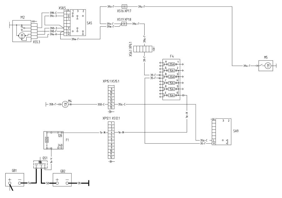
Connection diagram of the wind- and rear screen wipers and windscreen washer  $$^{236}$$
