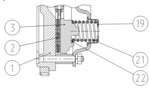
1 – flywheel; 2 – driven plate; 3 – pressure plate; 4 – PTO drive shaft; 5 – hub; 6 – power shaft; 7 – floating bushing; 8 – torsional vibration damper; 9 – clutch lever; 10 – backing plate; 11 – fork; 12 – nut; 13 – locking spring; 14 – bearing; 15 – shifter bracket; 16 – shifter; 17 – disengagement fork; 18 – control roller; 19 – sleeve; 20 – pressure spring; 21 – pressure spring; 22 – insulating washer.
