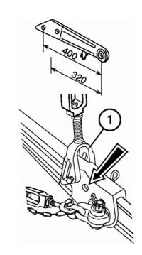
To increase the clearance when cultivating the high-stem crops, install the front ends of the lower rods onto the additional hanger axles located at the distance of 110 mm above the lower rod axis. To imitate field profile crosswise when operating wide-cut implements, connect the angle braces (1) with lower rods (2) via longitudinal grooves.
