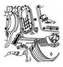
FDA number (on the right-hand sleeve at the front of the FDA (822) or on the central housing at the front of the FDA (72)).
