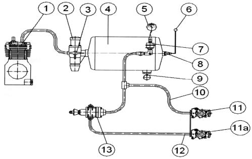
1 – compressor; 2 – pressure regulator; 3 – air intake valve; 4 – tank; 5 – pressure indicator; 6 – emergency pressure pilot lamp; 7 – pressure transducer; 8 – emergency pressure drop sensor; 9 – condensate removal valve; 10 – supply line; 11, 11a – connecting heads; 12 – control line; 13 – brake valve.
