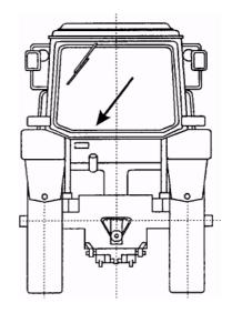
The serial number of the tractor is replicated on the front end of the right-hand side member of the half-frame (on the right plate of front balance weights).
