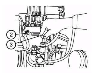
**NOTE:** If the engine starting is impeded, loosen the fuel line union nut of each injector and remove air from the lines by rotating the diesel engine with the starter. Rotate the engine for 10...15 s and then tighten the union nut.
