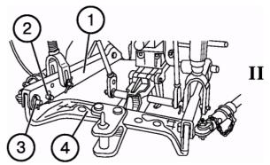
**IMPORTANT!** Make sure that the traction hitch mechanism is locked against lateral swinging by adjusting the internal or external tie bars.
