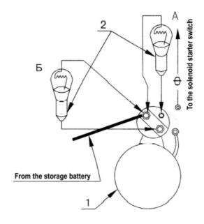
Fig.5. Checking the integrity of the windings of the solenoid starter switch "M3".
