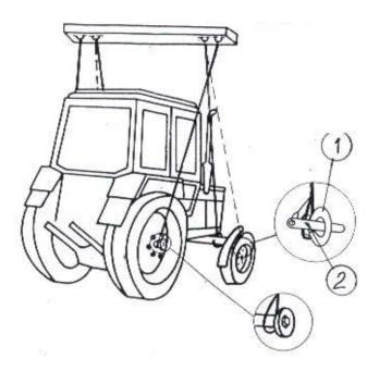
The ropes should be fastened at the front axle beam or eye-nut (1) and at the half-axles of the rear wheels as shown in the diagram below. When fastening the ropes by the eye-nut (1), draw the harness onto the eye-nut body and fix it by means of a stopper (2) through the eye of the eye-nut.
