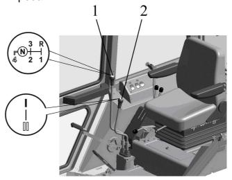
**ATTENTION:** When operating the tractor, do not hold the foot on the clutch pedal. It will prevent the clutch slip, which causes the overheating and premature failure of the clutch.
