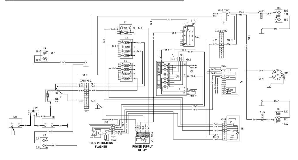
Diagram of the turn indicators and fault signalling
