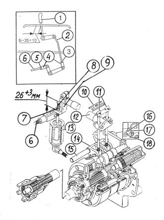
If the adjustment is made properly, the lever (1) in position "ON" will be at the distance of at least 35 mm from the control panel slot edge and will be neatly pass through neutral position (dead centre).
