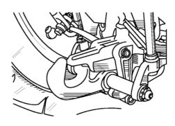
**Traction hitch mechanism TCY-1M** (floating lever): to operate with heavy trailing machines (optional). A combined variant with a hook for working with the semitrailers.
