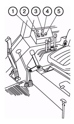
• "DL ON forcedly" – by pressing the lower part of the key (1). Fixed position. It is to be used for locking shortly the rear wheels when overcoming the obstacles. On releasing the lower part of the key, it returns to the mid position. On activating the DL, the pilot lamp (2) lights up, which becomes dim when unlocking the DL in the automatic mode and on setting the key (1) to the mid position.
