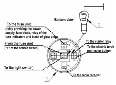
Fig. 9. Checking the operability of the starter switch (SA6). For the dashboard 826-3805010.
