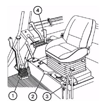
To unlock the hitch, lift the implement and turn lever (2) to the right.
