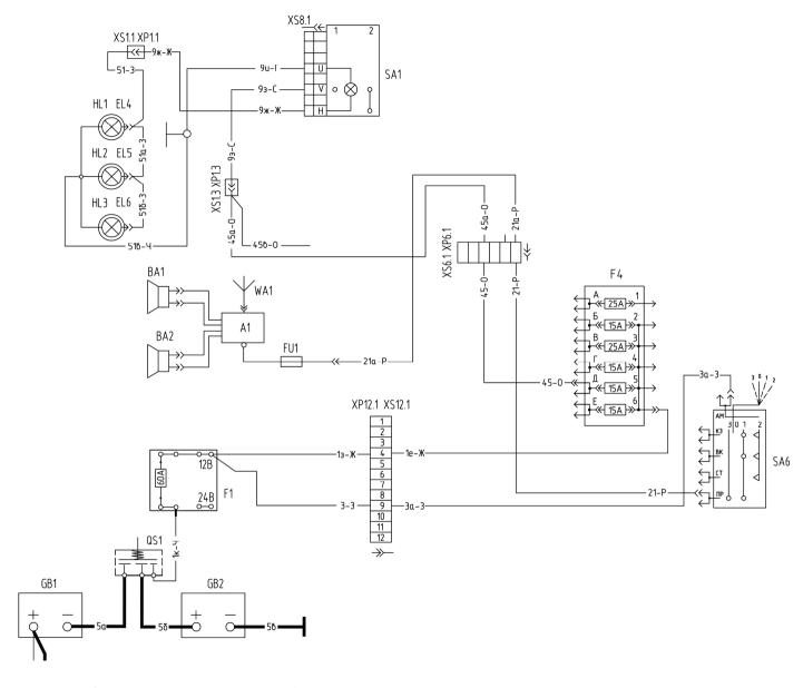
Connection diagram of the road train sign lights and radio equipment
