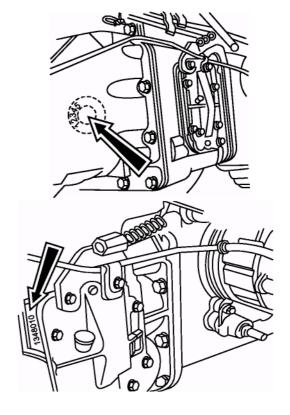
Gearbox number (on the left of the gearbox housing)
