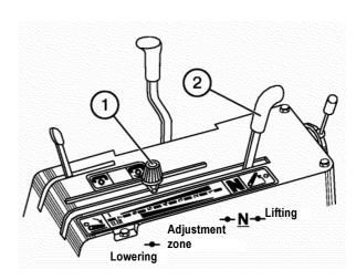
At the beginning of each run, lower the implement by pushing the handle (2) forward to the stop against limiter (1).
