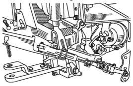
Traction hitch mechanism ТСУ-3К (trailer gear with automatic hitch): to operate two-axle trailers.
