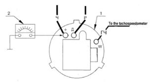
Fig. 1. Checking the controllable voltage value: 1 – alternator G1; 2 – voltage indicator.
