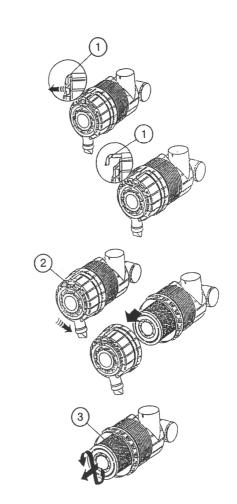
• Check the presence of clogging the filtering element (RFE) without removing it from the casing.
