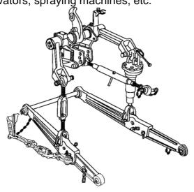
**Traction hitch mechanism (cross-bar) TCY-1X:** to work with trailing machines, potato combines and others (except single-axle ones) with the speed of up to 15 km/h.
