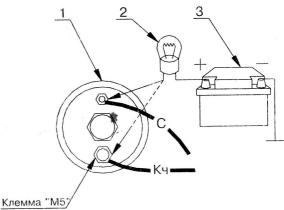
Fig. 14. Checking the operability of the electric torch pre-heater A2.
