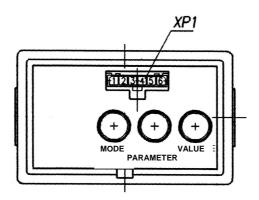
The programming board makes it possible to perform the manual programming of the combined indicator by means of the "Parameter" (Параметр) and "Value" (Значение) buttons and to modify the mode of display of the parameters to be shown on the LCD.
