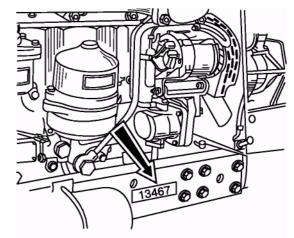
Engine number (is duplicated on engine name plate attached on the right of the cylinder block).
