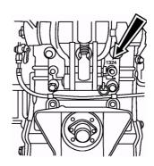
Transmission number for the tractor with hydraulic lift (on the rear axle housing at the joint with the gearbox on the right).
