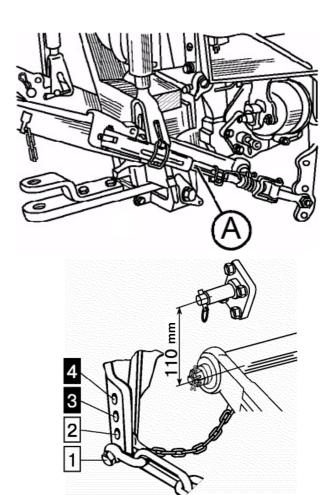
**ATTENTION!** The tie bars shall be installed only into the second from bottom apertures for holders (position 2) to avoid tie bar failure.
