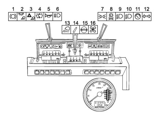
Three electric circuit fuse boxes are installed in the dashboard. To get access to the fuses, remove the screw on the dashboard cover and open it.
