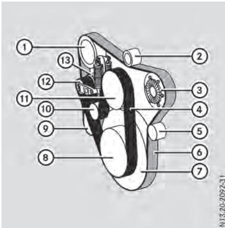
Engine with a dual-belt system (high-set fan)
