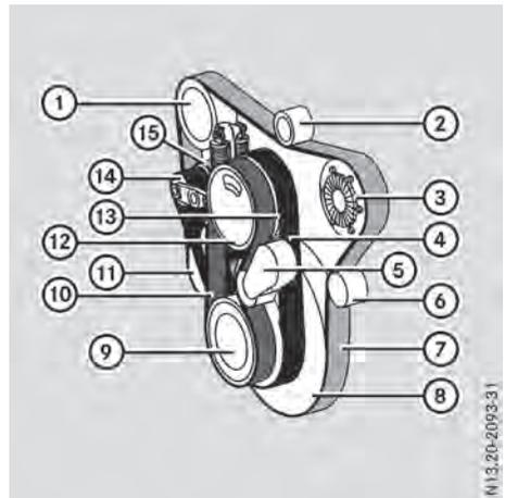
Engine with triple-belt system (fan on crankshaft)
