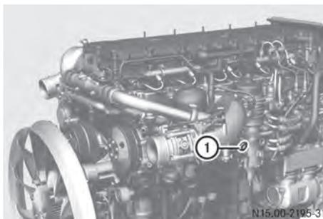
You can start and switch off the engine using the external engine start/engine stop button.
