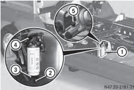
Example: fuel prefilter on the chassis frame
