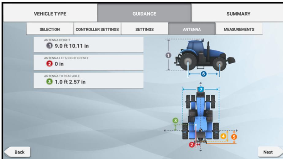
2. In the Vehicle Guidance - Measurements screen, enter values for the following measurements:
