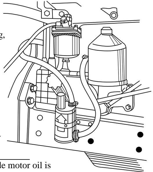
**NOTE:** The circulatory heater of coolant should only be used for cooling circuits filled up with antifreeze.
