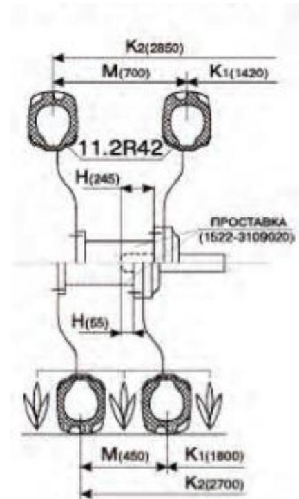
A spacer 1522-3109020-01 is used for inter-rows of 450 mm and 700 mm; the spacers for other inter-rows width are developed and shipped by a buyer's request (optional).
