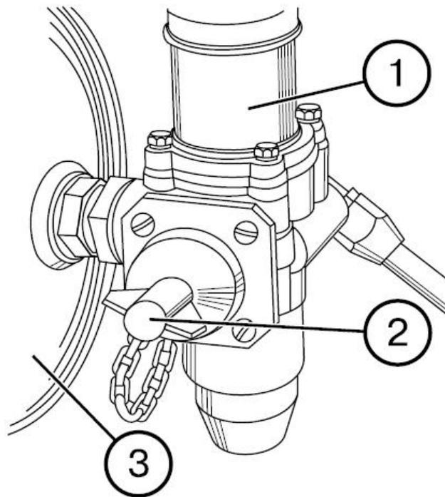
**IMPORTANT!** If pressure in a balloon exceeds  $7,7 \text{ kgf/cm}^2$ , the compressor is switched over to idling by a pressure regulator and tires inflation stops automatically. Thus, control a pressure level by an indicator on the dashboard and decrease pressure through a condensate ejection valve if necessary.
