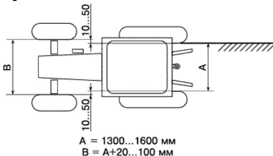
To obtain a tread size, add a profile width of a relevant tire to A and B sizes.
