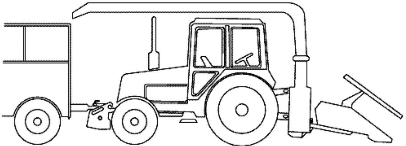
Driving on the roads of general purpose is performed only at forward motion. The motion on reverse is not permitted as signaling and lighting equipment is designed only for forward motion.
