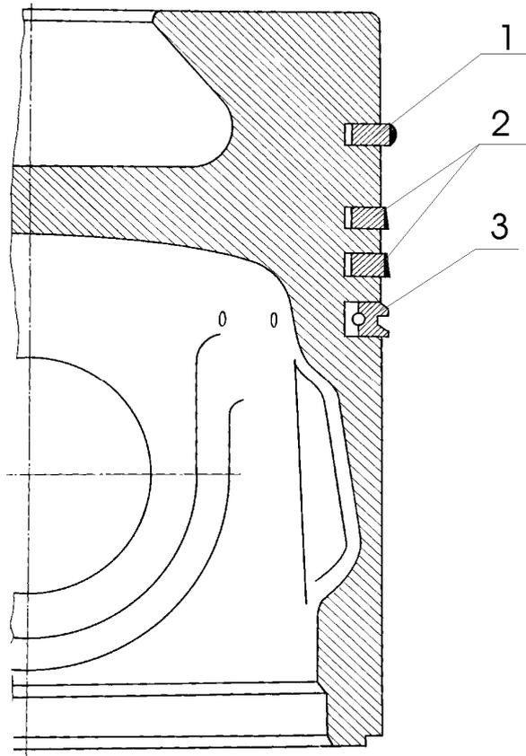
1 – upper compression ring; 2 – conic compression ring; 3 – oil ring.
