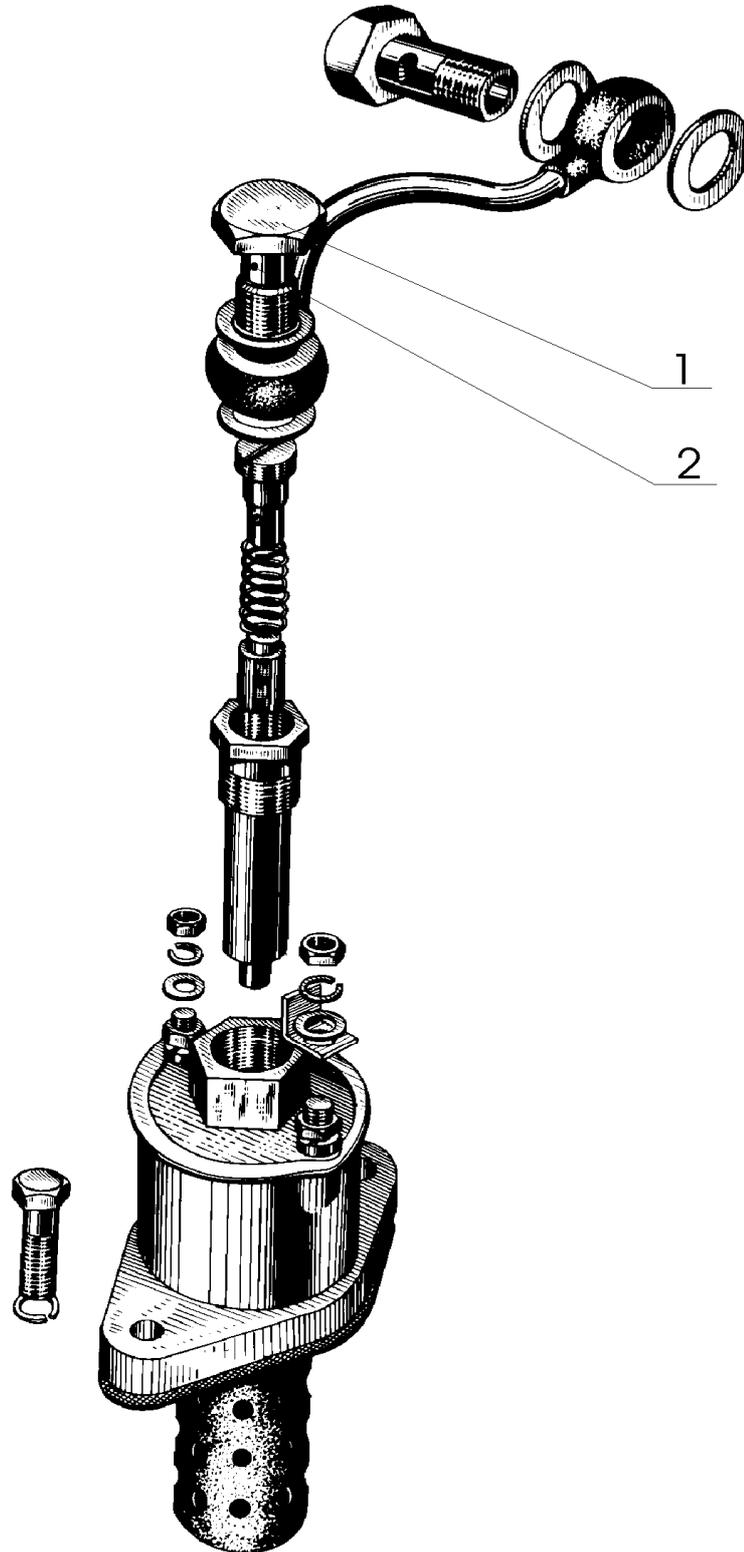
1 – pipe connector bolt; 2 – hole
