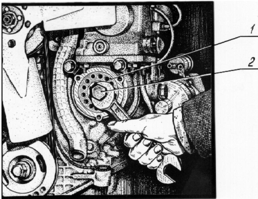
1 – slotted flange of the pump gear; 2 – fuel pump shaft nut.
