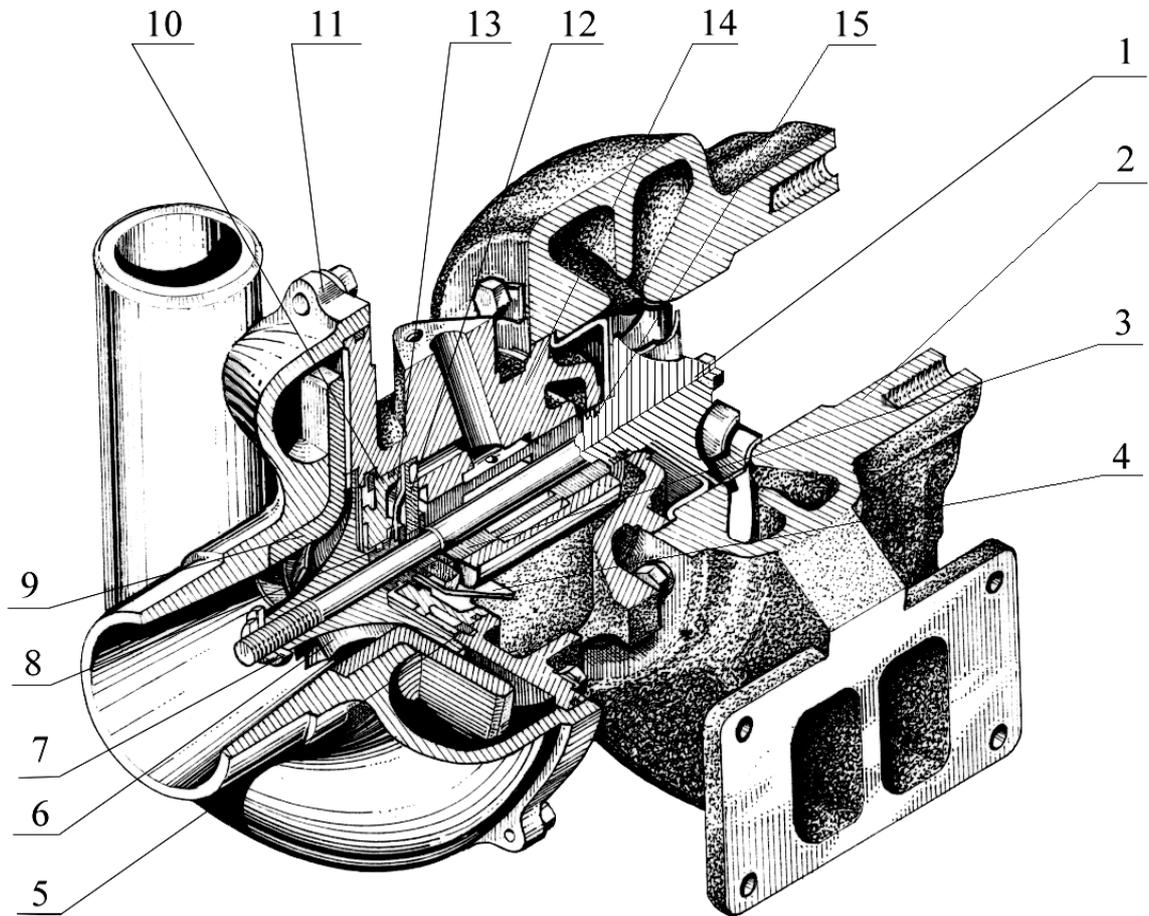
1 – turbine wheel with shaft; 2 – turbine housing; 3 – mono-bush; 4 – oil-guard; 5 – eccentric ring; 6 – compressor wheel; 7 – special nut; 8, 15 – O-rings; 9 – diffuser; 10 – cover; 11 – compressor housing; 12 – thrust bearing; 13 – distance bush; 14 – middle housing (housing of bearings).
