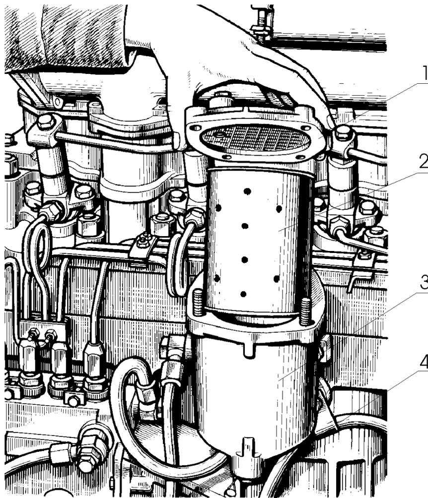
1 – filter cover; 2 – filter element; 3 – filter housing; 4 – plug.
