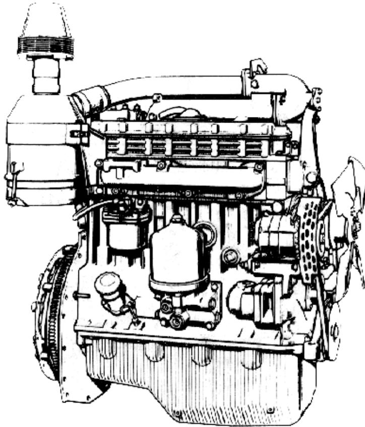
Fig. 3 – D-241 Diesel Engine (Right View).
