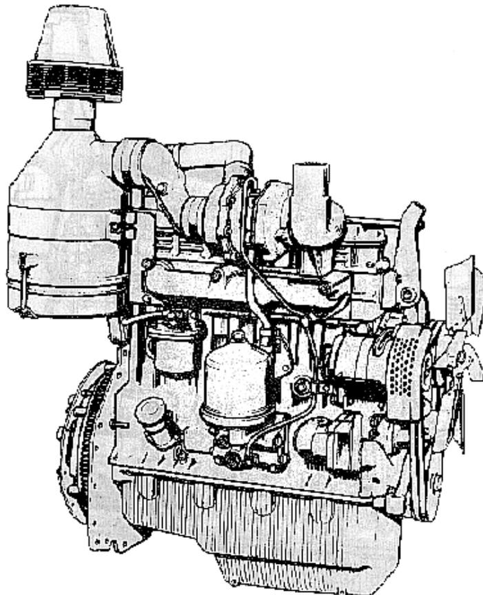
Fig. 6 – D-245 Diesel Engine (Right View)
