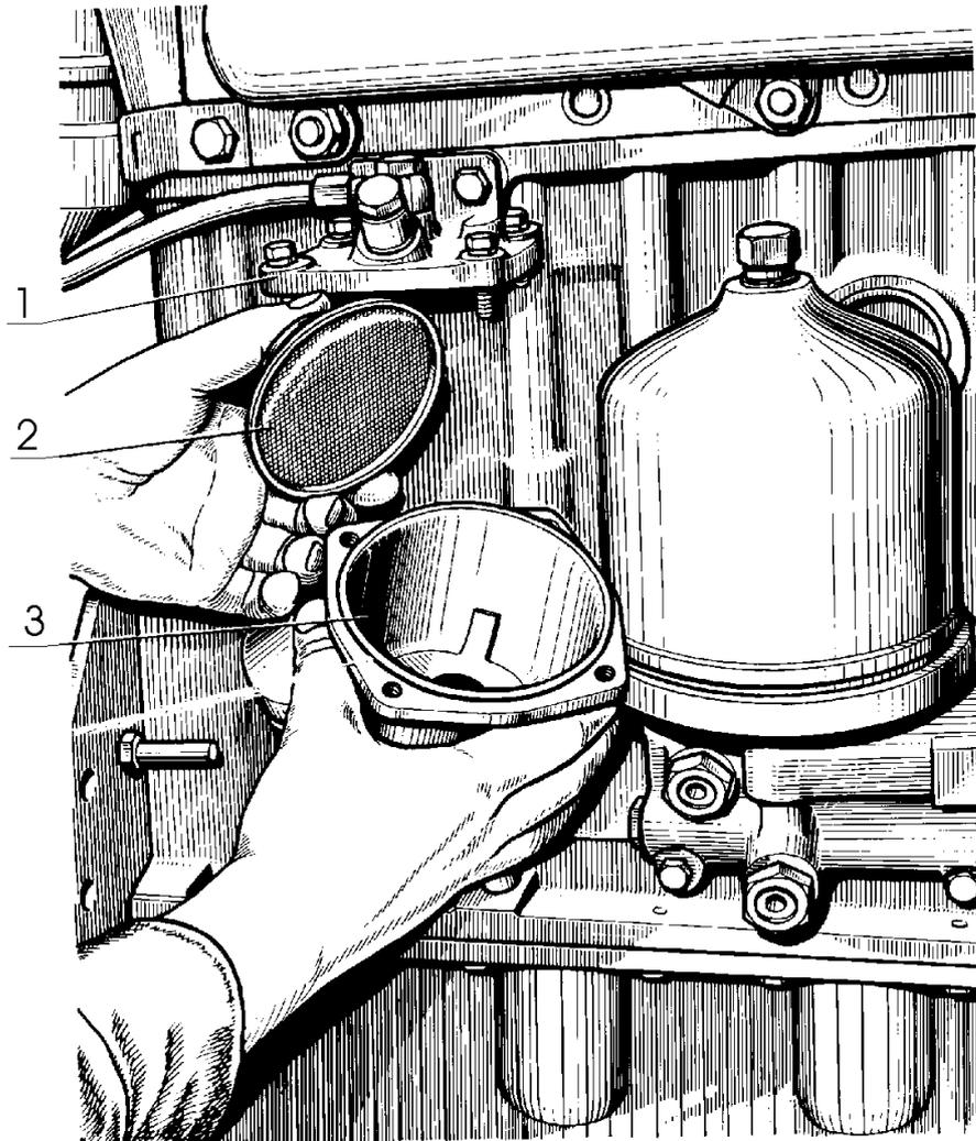
1 – filter housing; 2 – slinger with the filter screen; 3 – cup.
