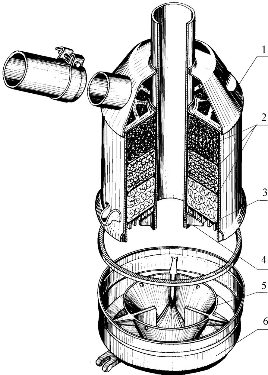
1 – air-cleaner housing; 2 – filtering elements; 3 – holder; 4 – holder stopper; 5 – oil reservoir; 6 – pan.
