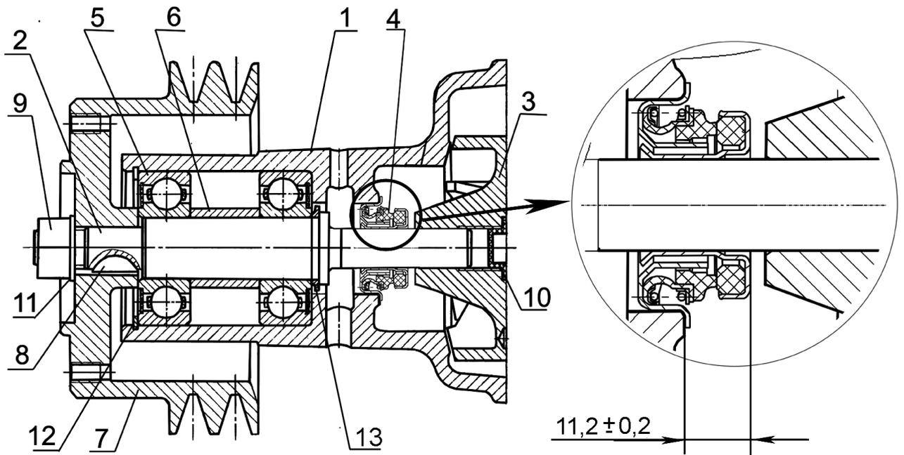
1 – Case; 2 – pump shaft; 3 – impeller; 4 – water pump sealing SP/1341; 5 – bearing; 6 – sleeve; 7 – sheave; 8 – dowel; 9 – nut; 10 – cap screw; 11 – washer; 12 – stop ring; 13 – sealing ring.
