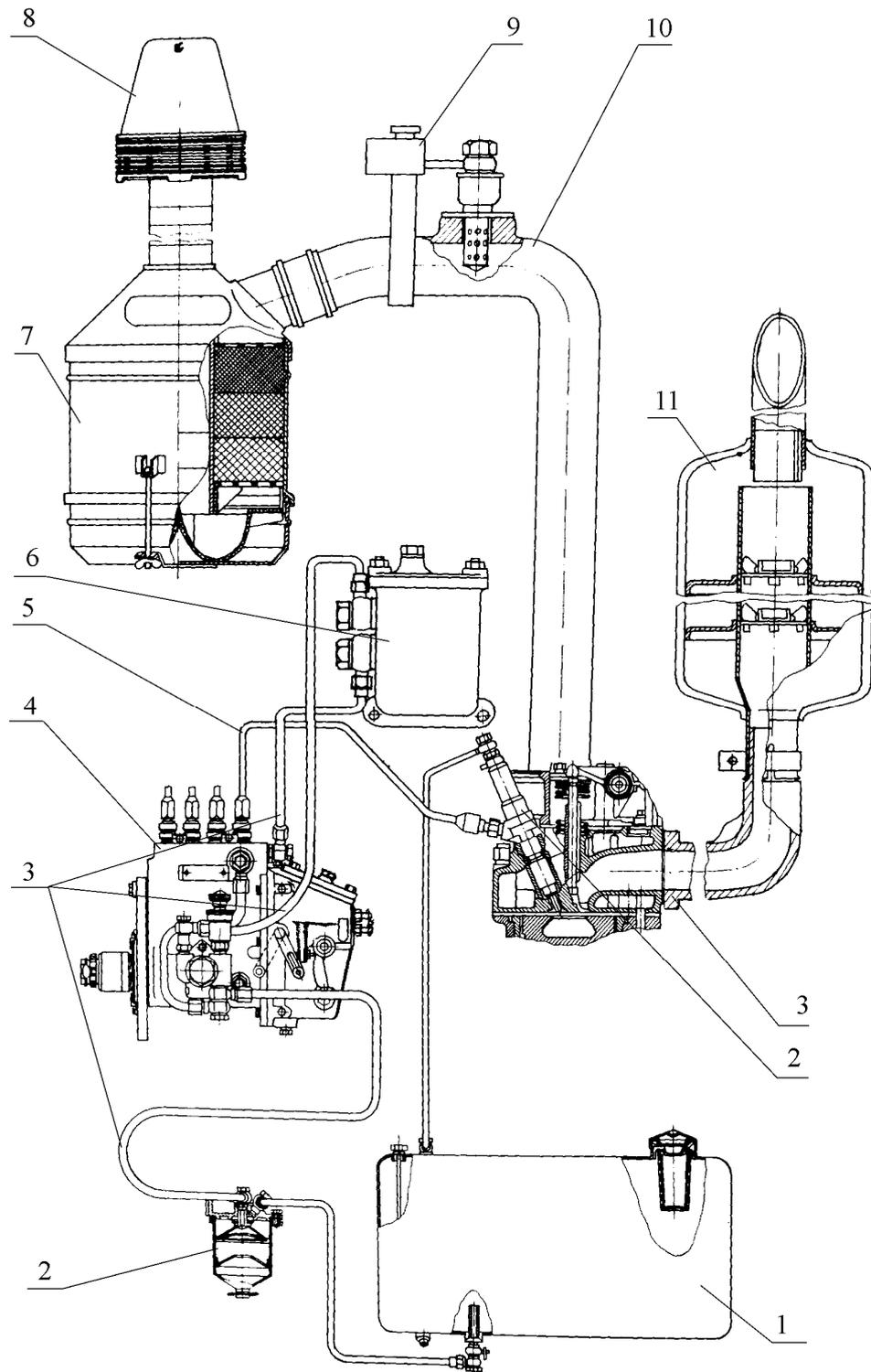
1 – fuel tank; 2 – coarse fuel filter; 3 – fuel pipes; 4 – fuel pump; 5 – high-pressure fuel pipe; 6 – fine fuel filter; 7 – air cleaner; 8 – coarse air filter; 9 – electric torch heater; 10 – intake manifold; 11 – muffler; 12 – exhaust manifold; 13 – fuel injector.
