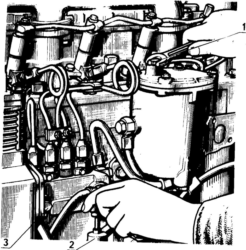
1 – fitting; 2 – priming pump; 3 – plug.
