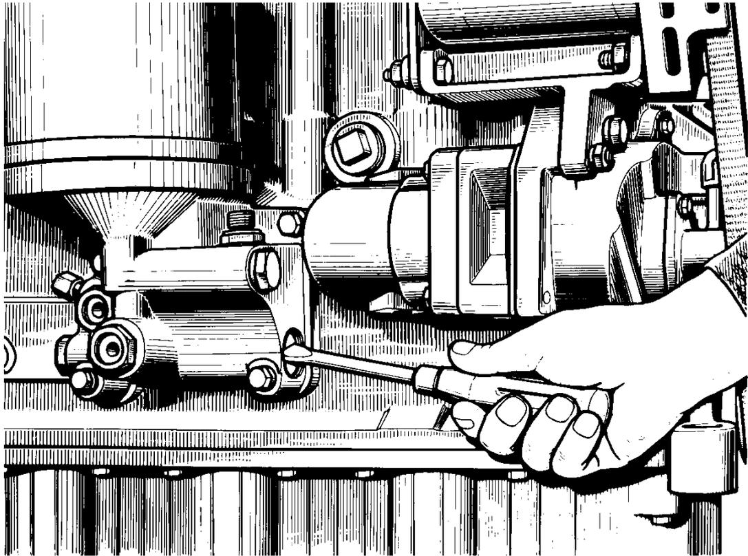
Fig. 17 – Adjustment of the draining valve of the centrifugal oil filter.
