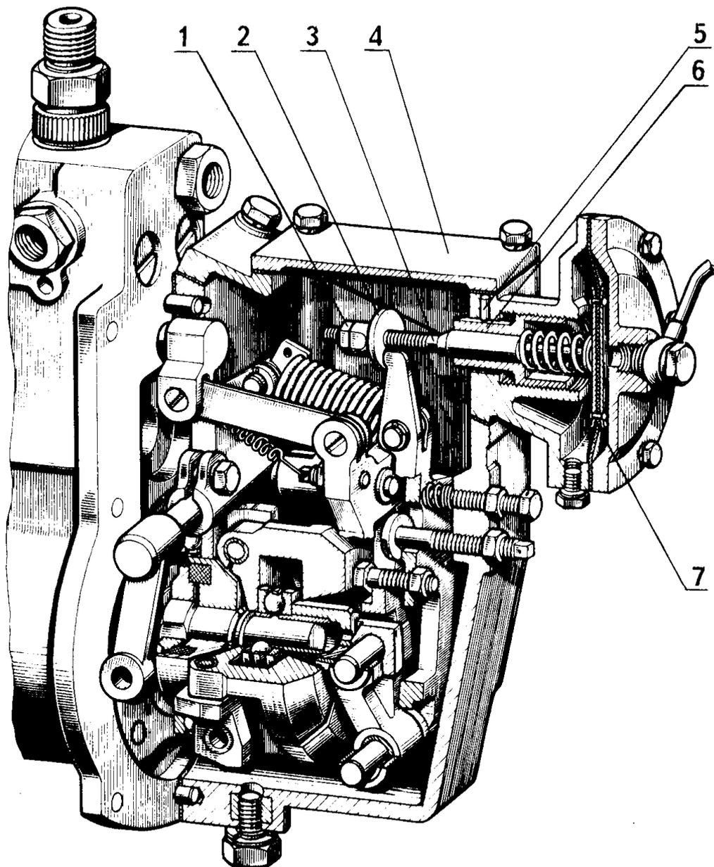
1 – lock nut; 2 – stop; 3 – rod; 4 – cover; 5 – dowel; 6 – bush; 7 – diaphragm.
