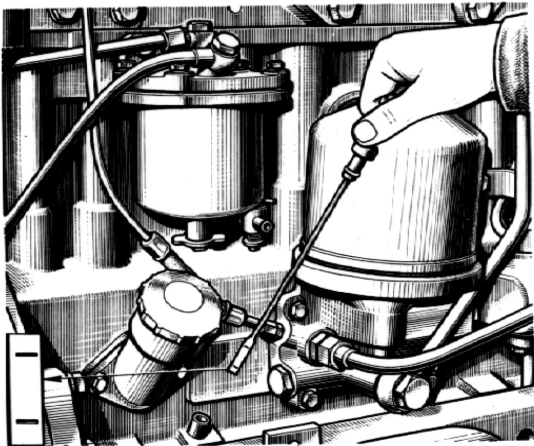
Fig. 12 – Checking the oil level in the diesel engine crankcase.
