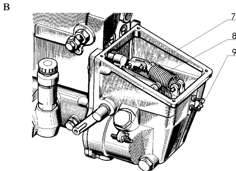
1 – adjusting screw; 2 – nominal bolt (stop); 3 – teeth crown; 4 – fixing screw; 5 – rotating bush; 6 – pusher adjustment bolt with lock nut; 7 – shackle; 8 – governor spring; 9 – idling spring adjustment bolt.
